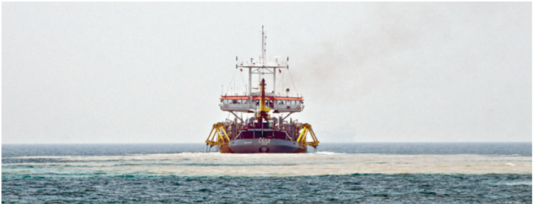
The Goryo 6 Ho Hyundai dredger was designed to suck sand from the seabed. Here, it operates near Nipah Island, Indonesia.
